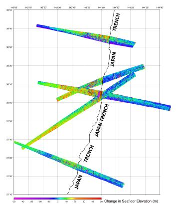
Figure 2. Results of five bathymetric surveys showing the differential bathymetry pre- to post-Tohoku 2011 (Fujiwara et al., in prep.) The resolution of differential bathymetry is around 20 m. The largest observed vertical motion occurred at around 38°N close to site C0019. Transects further north and south of 38°N are unable to resolve significant vertical changes, implying the changes are less than 20m.
