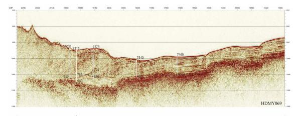
Figure 4 High-resolution seismic reflection survey through the Japan margin ~2 km south of the repeat bathymetry line at 38° 30'N. Estimated water depths and depths to prominent reflectors shown.
