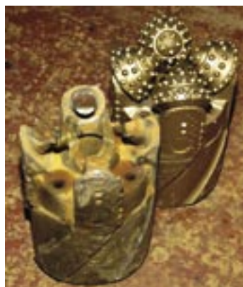
A completely destroyed C-7 drill bit rests next to a new one, demonstrating the hardness of the recrystallized dikes Expedition 312 drilling penetrated before reaching gabbros. (Photo: IODP-USIO/TAMU)
