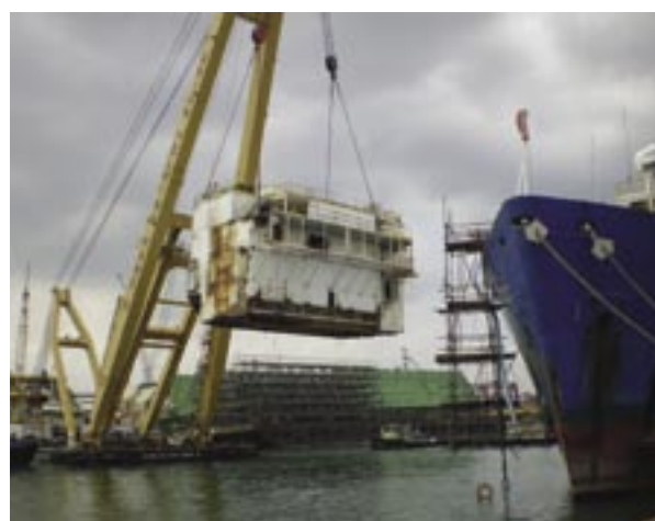
The labstack is removed from the JOIDES Resolution while it is at a shipyard in Singapore. (Photo: IODP/TAMU)
