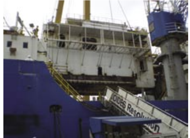
Once it was cut free, the labstack was lifted from the JOIDES Resolution. It was sold as unit to serve as living space in Thailand. (Photo: IODP/TAMU)
