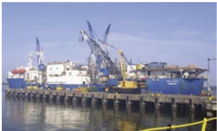
The derrick of the JOIDES Resolution has been removed and will be refurbished. (Photo: IODP/TAMU)
