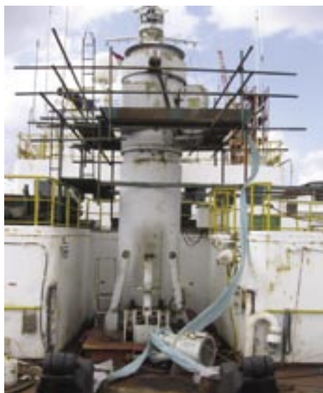
The forward bow thrusters were removed from the JOIDES Resolution to be updated and refurbished. (Photo: IODP/TAMU)
