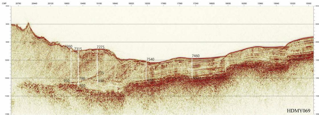
Figure 4 High-resolution seismic reflection survey through the Japan margin  $\sim 2$  km south of the repeat bathymetry line at  $38^{\circ} 30'N$ . Estimated water depths and depths to prominent reflectors shown.
