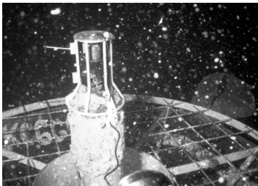
Fig. 2: Photograph taken from the Alvin submersible in 1993 showing a bacterial mat covering the data logger, which was bathed in hydrothermal fluid leaking from the bottom of the Hole 858G reentry cone. Subsequent observation of the hole with the drillstring TV camera prior to reCORKing on Leg 169 showed that the bacterial mat had disappeared and that hydrothermal venting had ceased sometime between 1993 and 1996.
