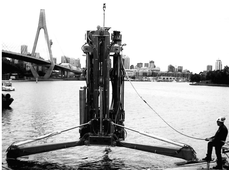
The PROD drill, operated by Benthic GeoTech Pty., Ltd., an Australian consortium, has the capability of penetrating to a depth of 100 m below the seafloor. It remotely assembles a drill string from joints stacked in rotary rack. It is 5.8 m in height, weighs 10 tons in air, and drills a 35-mm diameter core. Currently this drill is limited to water depths less than 2000 m.
