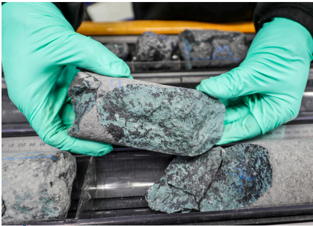
LEFT: Green alteration along a crack in a basalt core collected during Expedition 395C (Credit: Sarah Kachovich & IODP JR50). RIGHT: Competing hypotheses for V-shaped ridge (VSR) formation (Parnell-Turner et al., 2017). VST = V-shaped trough. (A) Thermal pulsing hypothesis (Vogt, 1971). (B) Propagating rift hypothesis (Hey et al., 2010). (C) Buoyant mantle upwelling hypothesis (Martinez and Hey, 2017).
