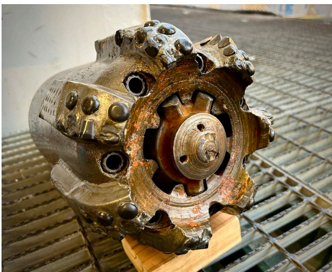
TOP: The contrast between a new center bit (left) and the one recovered from Hole C0019M (right) (Dick Peterse & JAMSTEC/IODP). BOTTOM: Chert – 1 point. Drill bit – 0 (Lena Maeda & JAMSTEC/IODP).
